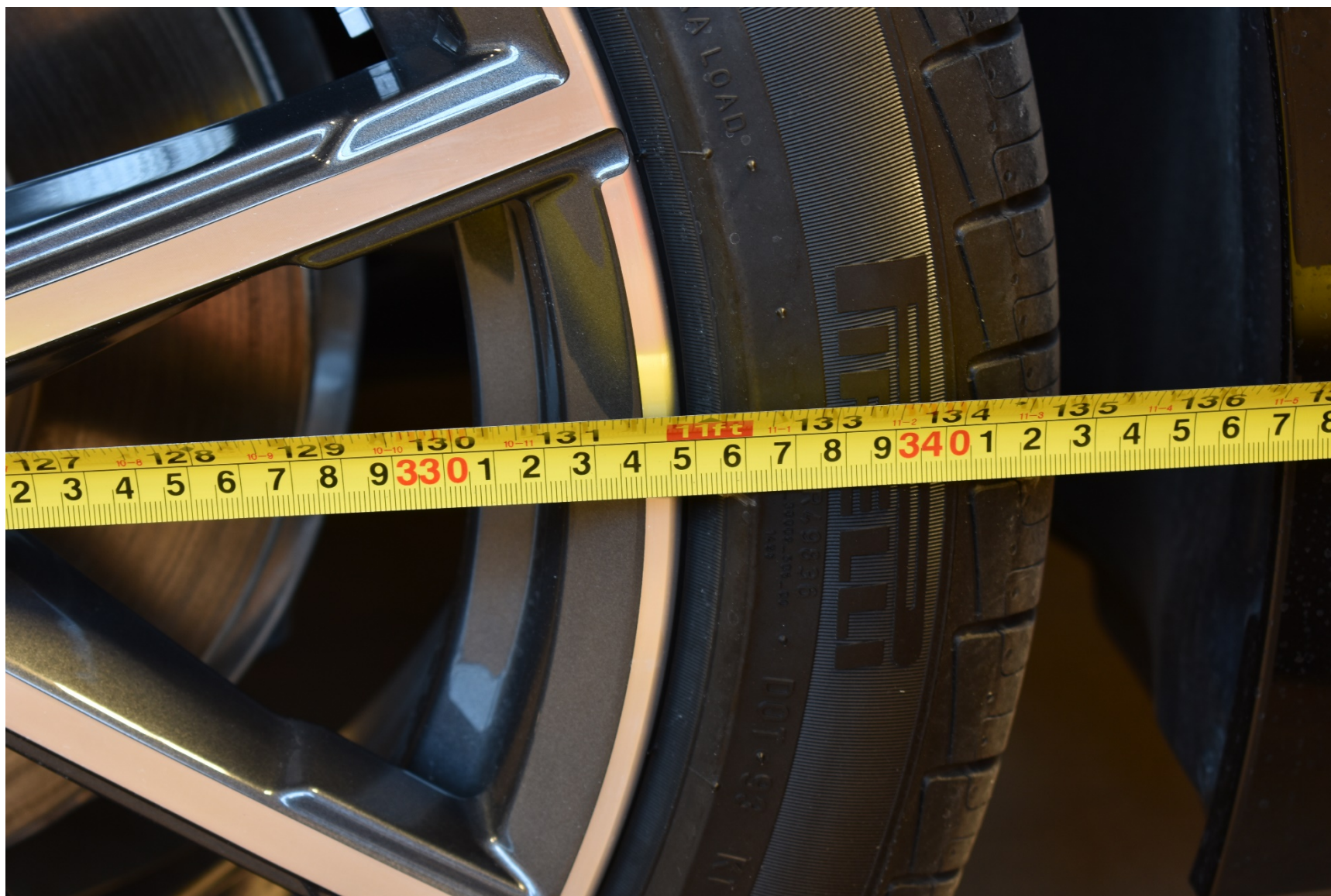
FIGURE 5.27 MEASURING VEHICLE RIGHT SIDE WHEELBASE OUTSIDE EDGE TO OUTSIDE EDGE
